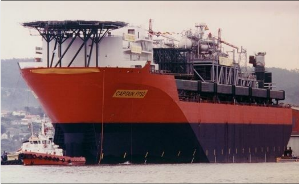
The Captain FPSO (floating production, storage and offloading ) Vessel after its launch
